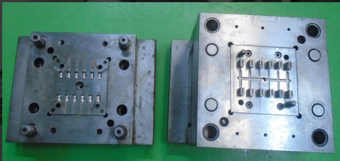
Mold for Housing Terminal Brush Free Yellow Tool Size in Inches : L 11" X W 8" X H 9"
